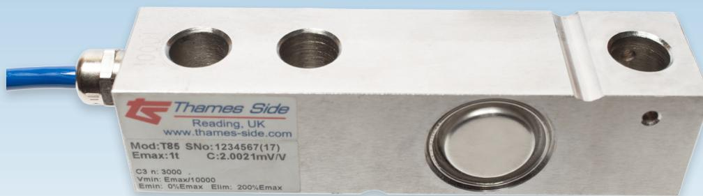
This stainless steel shear beam load cell is available with approval according to OIML R60 Class C3 (3000 divisions) and is calibrated in mV/V/Ω by output current matching, which minimises corner correction time on multi-cell systems.
